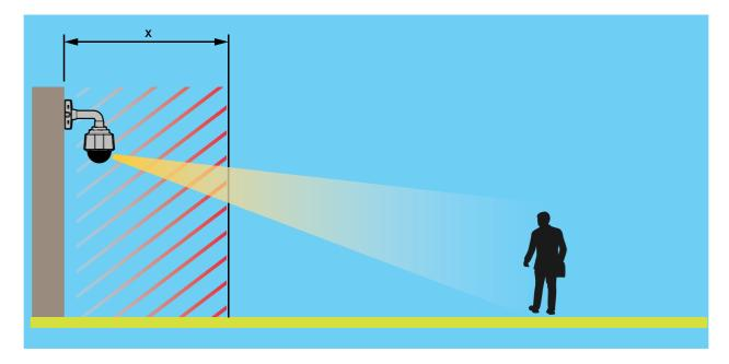
Move speed sets the speed of the camera's pan and tilt movements. The default setting is maximum speed.
