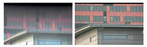
Figure 6: An image from a conventional dome (to the left) and Sharpdome (to the right) at a 20° tilt, 20× zoom.
