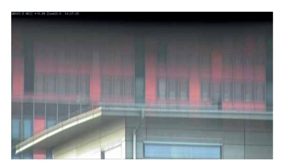
Figure 2: Mirroring in a conventional dome camera at 20° tilt, 20× zoom.
