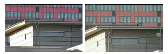
Figure 5: A conventional dome (to the left) and Sharpdome (to the right) at a 5° tilt, 20× zoom.
